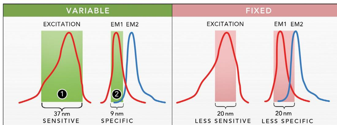
The plate reader optics of Cytation use a quad monochromator design with variable bandwidth. The bandwidth can be set anywhere between 9 and 50 nm in 1 nm increment. Large bandwidth settings (1) provide increased sensitivity and lower limits of detection. Small bandwidth settings (2) provide increased specificity when multiple signals are present, which reduces signal crosstalk and enhances assay performance.
