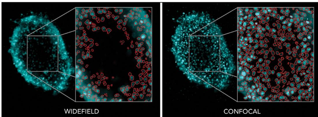
Confocal microscopy can enable you to see a level of detail in your samples that is not possible with widefield optics. Not only can you obtain improved image quality, you can get improved quantification and analysis with confocal images and Gen5 software.
