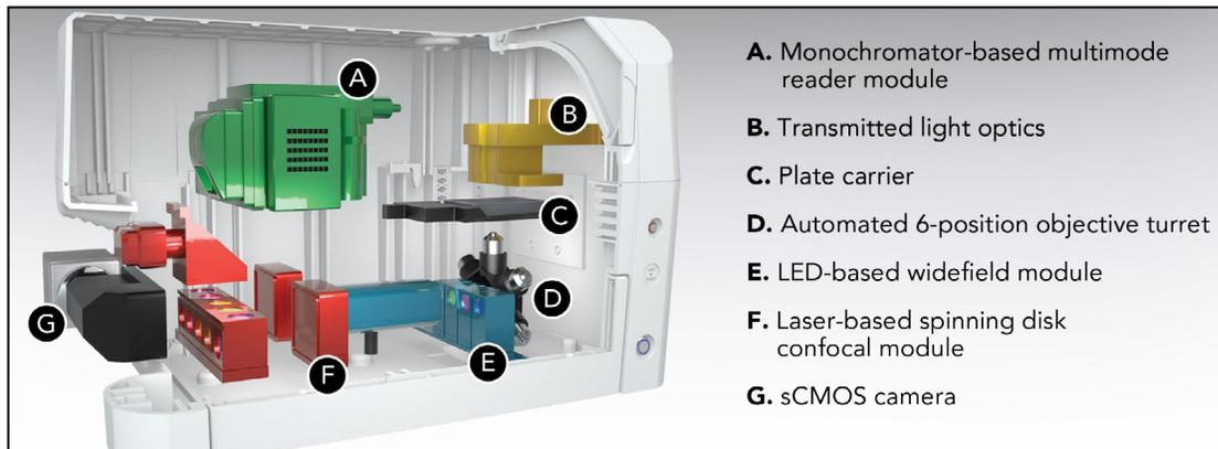
With a combination of spinning disk confocal and widefield imaging, plus multi-mode reader, Cytation C10 is truly ready for any assay. And since Cytation C10 is a modular, upgradable instrument, you can get the functionality you need today and add modules later as your needs expand.
