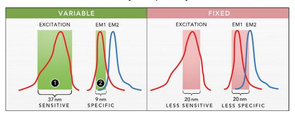
The plate reader optics of Cytation use a quad monochromator design with variable bandwidth. The bandwidth can be set anywhere between 9 and 50 nm in 1 nm increment. Large bandwidth settings (1) provide increased sensitivity and lower limits of detection. Small bandwidth settings (2) provide increased specificity when multiple signals are present, which reduces signal crosstalk and enhances assay performance.
