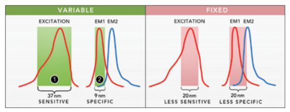
The plate reader optics of Cytation 7 uses a quad monochromator design with variable bandwidth. The bandwidth can be set anywhere between 9 and 50 nm in 1 nm increments. Large bandwidth settings provide increased sensitivity and lower limits of detection. Small bandwidth settings provide increased specificity when multiple signals are present, which reduces signal crosstalk and enhances assay performance.
