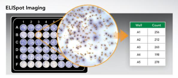
Cytation 7's upright imaging module can be used to automate assays such as ELISpot, in which cell secretions are rendered visible through the use of a colorimetric reaction. Cytation 7 fully automates image acquisition, processing, image analysis and object count.
