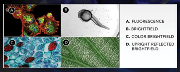
Cytation 7's inverted microscopy module supports fluorescence, brightfield and color brightfield from 1.25x to 60x to analyze both large objects and intracellular details.
