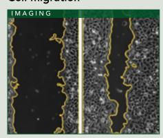
High throughput cell migration assays are enabled with AutoScratch Wound Making Tool, with time-lapse imaging under environmental controls in Cytation 7.
