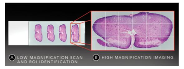
Cytation 7 and Gen5™ software facilitate ROI identification. Cytation 7 scans samples at low magnification before prompting the user to identify regions of interest to be imaged at high magnification. This greatly accelerates the process of imaging ROIs in batches of complex microscopic samples.
