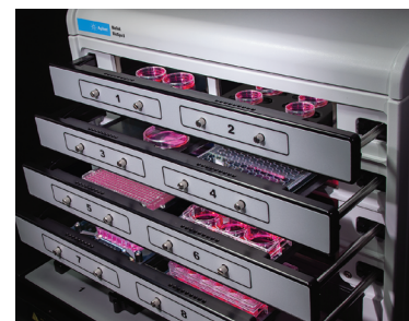
The Agilent BioTek BioSpa 8 automated incubator processes up to eight microplates or other labware at a time.
